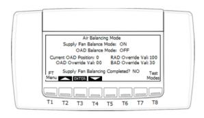
Figure 2. i-Controller Air Balance Mode - Supply Fan
