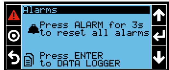
Figure 91. Alarms Reset Screen
