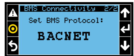
Figure 77. BMS Config Screen 2
