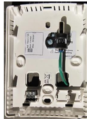
Figure 4.3. 501-1125 Temp Sensor Mounting Position In RH
