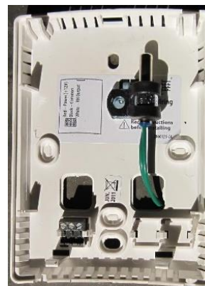
Figure 4.3. 501-1125 Temp Sensor Mounting Position In RH
