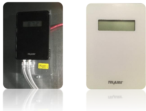
Figure 5. CO2 sensor located inside unit
