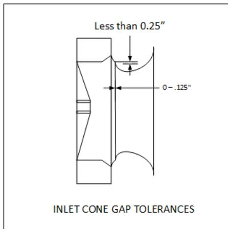
Figure 20. Supply Fan Inlet Cone Tolerances
