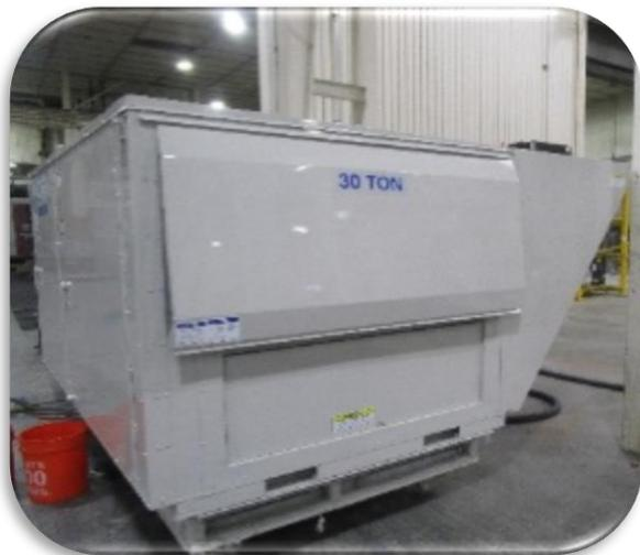
Figure 3. Small Unit - Closed Air Hood
