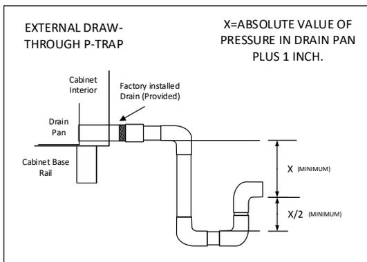
Figure 12. External Draw-through P-Trap
