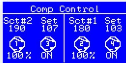
Figure 6. Compressor Control Screen
