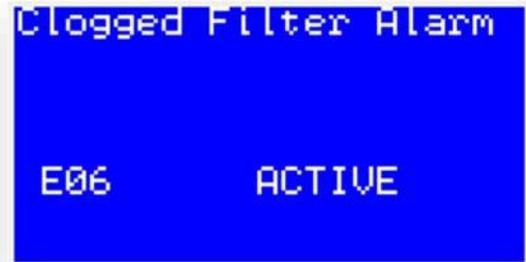
Figure 10. Active Clogged Filter Alarm
