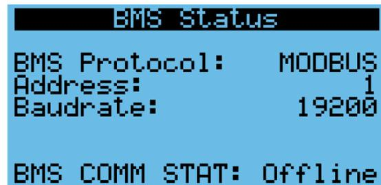
Figure 1. i-Controller BMS Status screen
