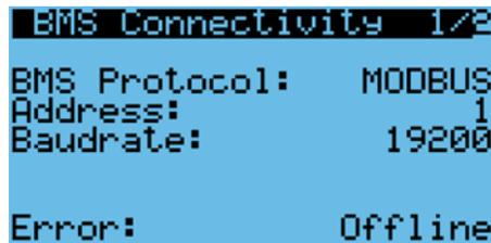
Figure 2. i-Controller BMS Configuration Screen 1
