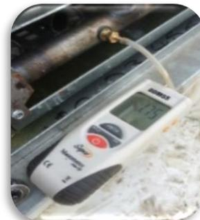
Figure 2. Manometer Connected to Gas Port
