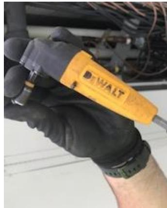
Figure 20. 90-Degree Adapter
