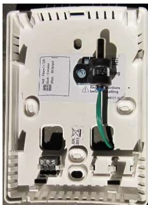
Figure 5.3. 501-1125 Temp Sensor Mounting Position In RH
