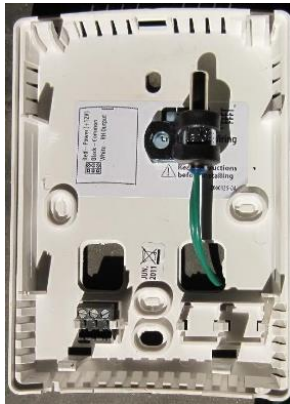
Figure 5.3. 501-1125 Temp Sensor Mounting Position In RH
