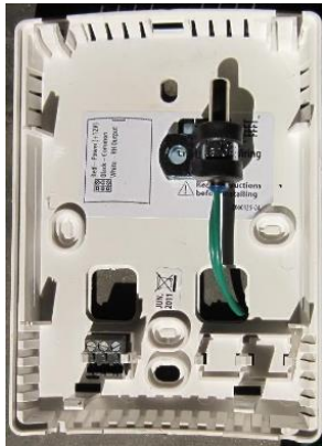
Figure 5.3. 501-1125 Temp Sensor Mounting Position In RH
