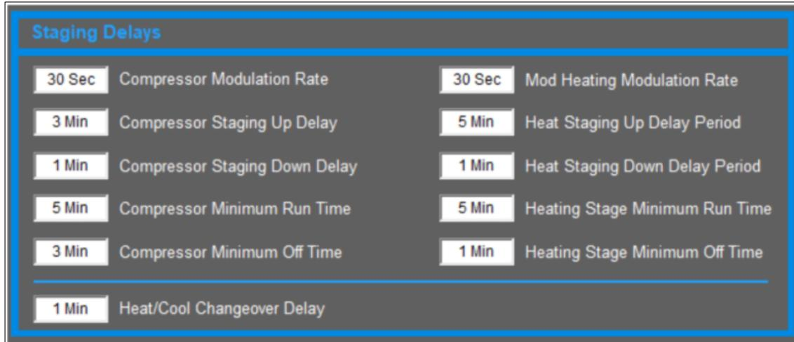
Figure 42: VCCX Staging Delays Category Example (Do Not Use This Example To Configure Your VCCX)
