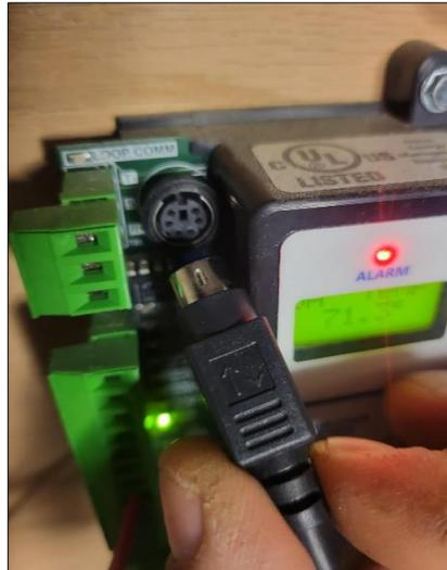
Figure 19: VCCX Plug Orientation
