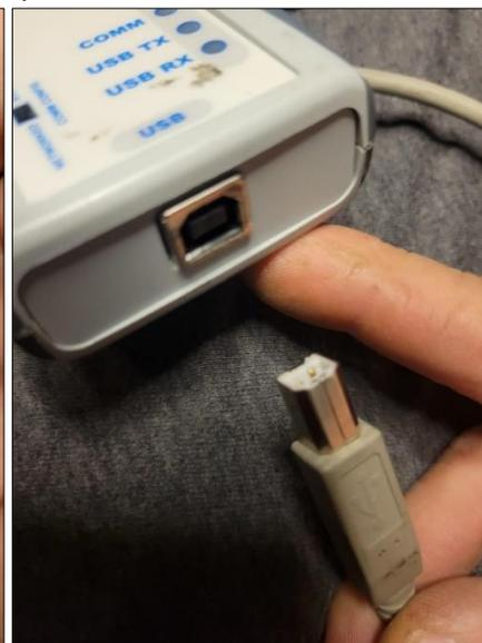
Figure 21: RS-485 Cable Connection To USB Link 2
