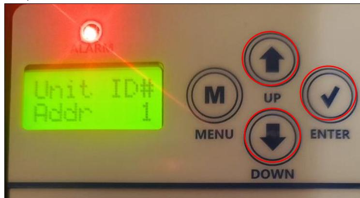
Figure 47: Setting The Unit ID On VCCX
