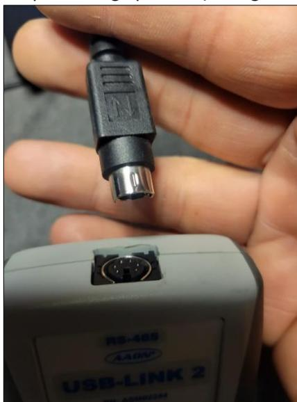
Figure 20: Pinned Connector Cable Connection to USB Link 2
