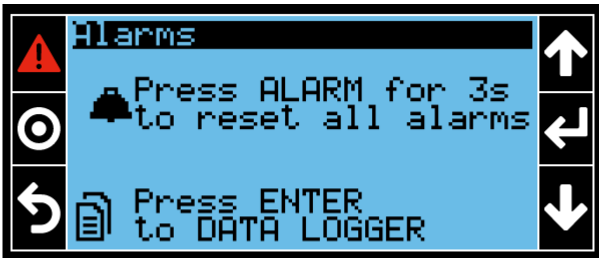
Figure 109. Alarms Reset Screen
