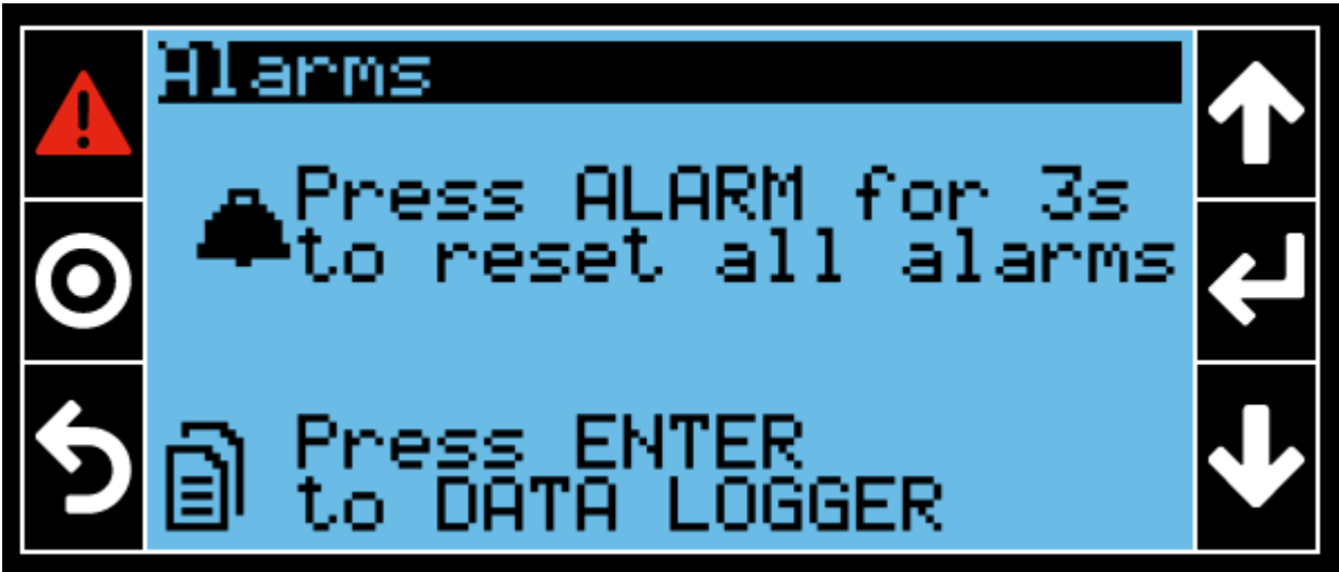
Figure 110. Alarms Reset Screen
